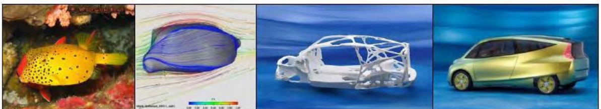
Figure 4: DaimlerCrysler bionic car inspired by the box fish and tree growth patterns. (Source: Pedersen Zari, M. 2007).
