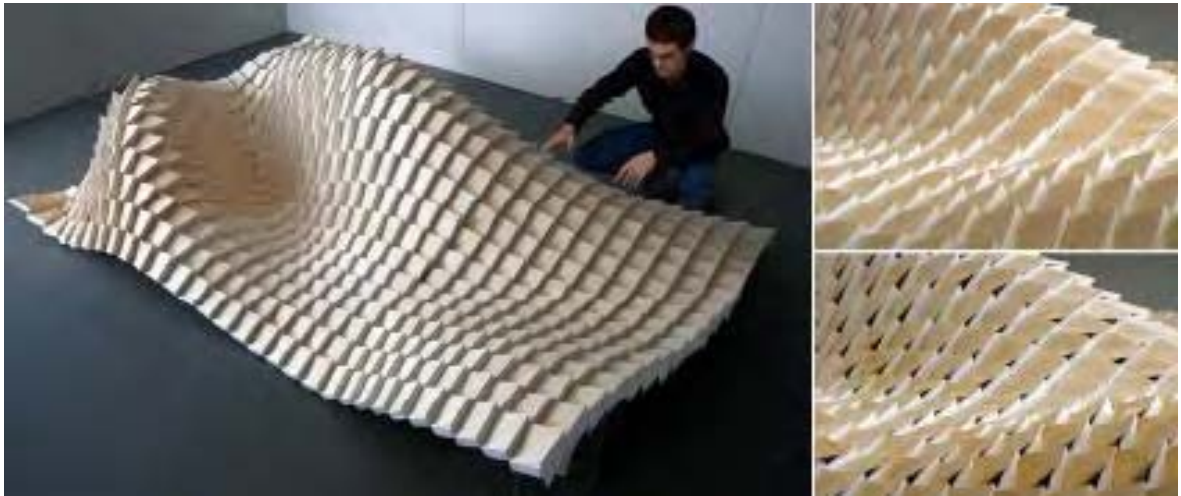
Figure 49: Functional Prototype of responsive surface (left) with Responsive Veneer Skin (right). (Source: Hensel M. 2009).
