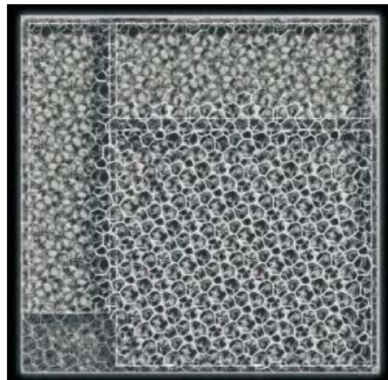
Figure 22: Watercube digital structural model. The mathematics of foam geometries are used to produce the structural array, ensuring a rational optimised and buildable structural geometry. (Source: AD Journal, Volume 76 no.4, 2006.)
