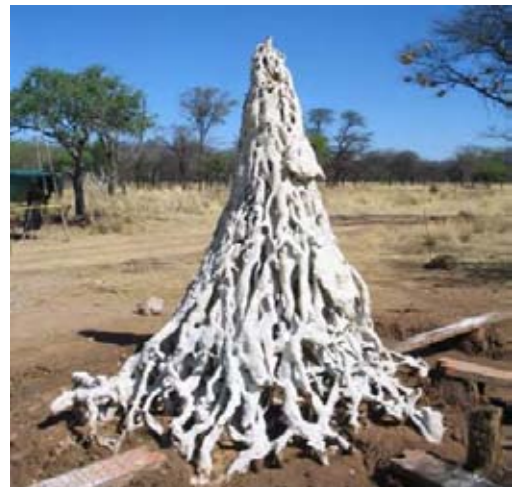
Figure 43: Plaster cast of ventilation chambers of a termite mound.
