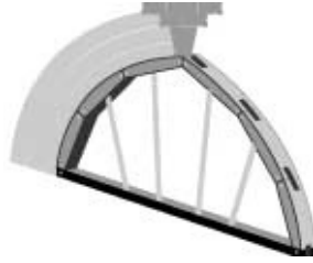
Wooden centering supporting an arch.
