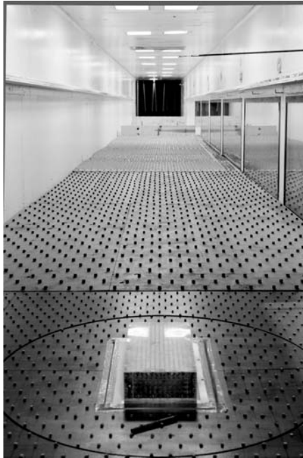
Figure 13.3.1. Meteorological wind tunnel, Wind Engineering Laboratory, Colorado State University. Model and turntable are in the foreground, and spires are in the background (courtesy of Professor Bogusz Bienkiewicz; photo by Gregory E. Stace).
