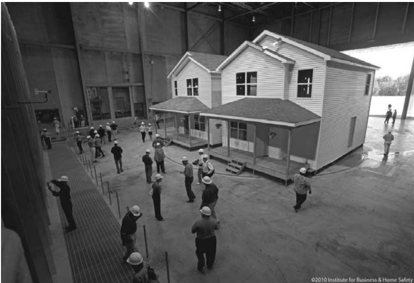
Figure 13.3.5. Interior view of IBHS Research Center with full-scale specimen, placed on the 55-foot diameter turntable with a surface area of 2,375 square feet. The 105-fan array with 300 hp motors is located to the left of the picture. (Courtesy of the Institute for Business & Home Safety.)
